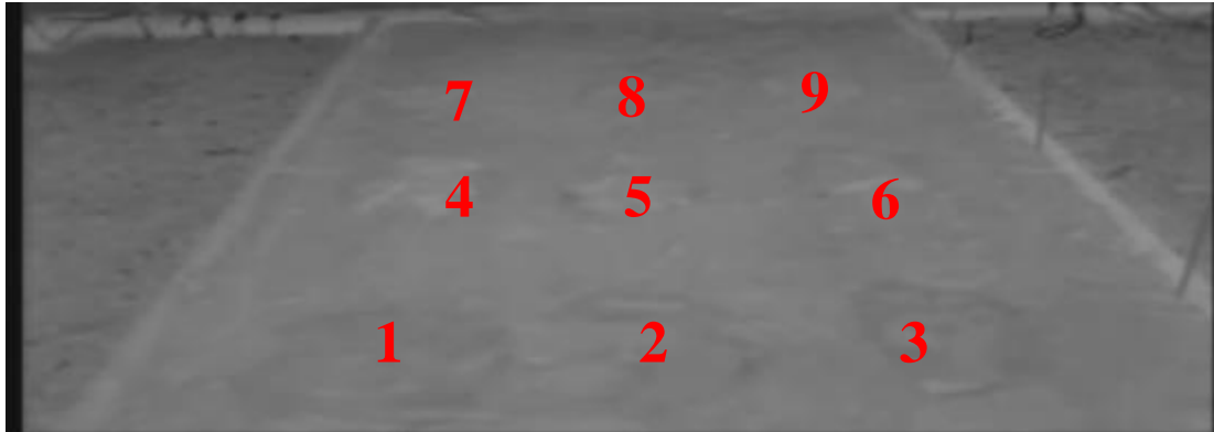
Figure 5: A scenario for target detection based on temperature and depth. Holes were dug at 5cm, 10cm and 15cm on a rather cold day (5 degrees). Then, landmines were placed on the first six holes, and the last 3 holes were covered up without placing anything in the hole. (1) Cold landmine placed at 15cm, (2) cold landmine at 10cm, (3) cold landmine at 5cm, (4) warm landmine at 15cm, (5) warm landmine at 10cm, (6) warm landmine at 5cm, (7) blank hole at 15cm (disturbed earth), (8) blank hole at 10cm and (9) blank hole at 5cm. Cold landmine is a landmine that was at the outside temperature, whereas a warm landmine has been recently buried after being at room temperature.
