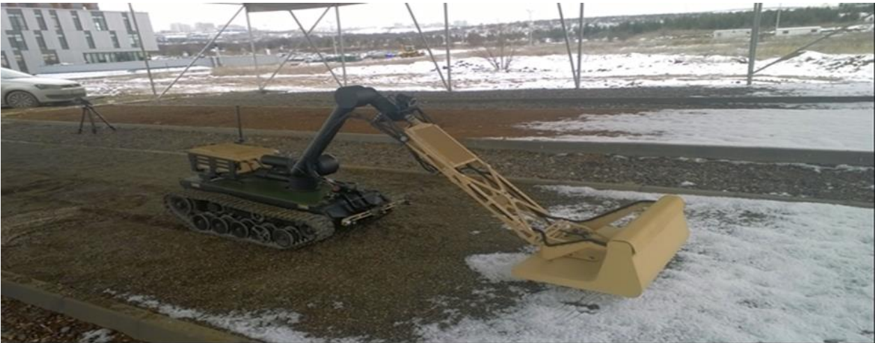
Figure 1: GPR, thermal and visible cameras mounted on a robot and scanning the lanes with varying soil content.
