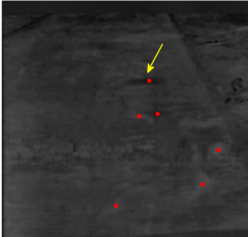
(a) FL-LWIR results: the dark region indicated with the yellow arrow is the location of the landmine. Red points are the alarms found by local RX.
