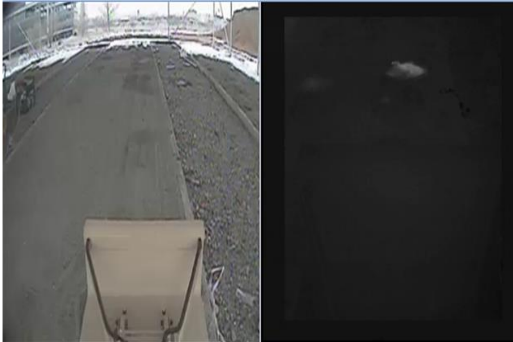
Figure 2: The scene of data collection from the visible camera on the left, and from the thermal camera on the right. In the thermal image, disturbed earth appears to have a lighter color.
