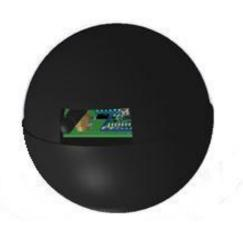
The outer shell of the device is designed to be like a tennis ball. When necessary equipment was found in this sphere, the diameter of the device was calculated as 10.5 cm. The designed device
