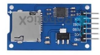
The increasing bandwidth, lowers the range. Since Lora has long range connection, the data size it can send in one packet is small. The main problem was sending large-sized data such as image. So we need the sd card to send these data.
