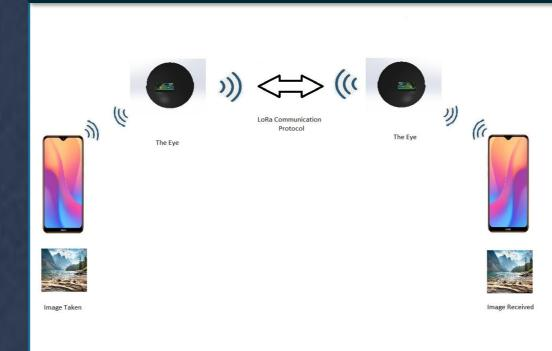
User can send an image, GPS location or text message with using The Eye. If the message is an image, our app The Eye changed the jpeg format into Base64. Then sends it to microcontroller at the
