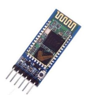
In order to provice communication between the Eye and a smartphone, HC05 bluetooth module was chosen because of its high speed.
