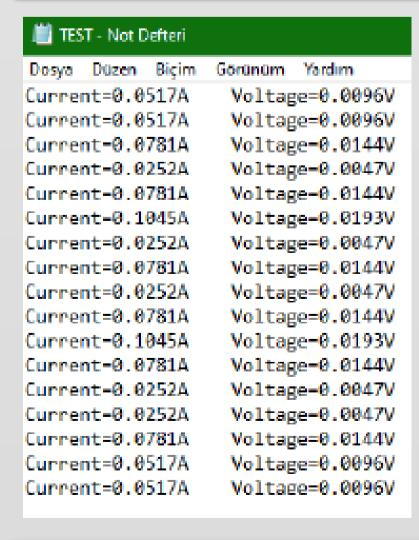
Applying this circuit as in the figure the current and voltage values was measured using current sensor in every 0.5 secs. and all data sent to the sdcard using MicroSd card module. MicroSd card create a text file and saved all data in it. Using that way it is observed that the current and voltage values when GSM/GPS vehicle tracking system is on.
