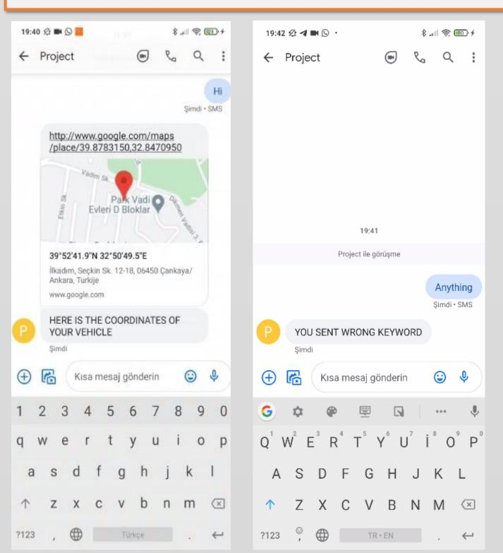
Here you can see the result of one of our tests. The responses, according to the correct keyword and a random message. The exact location of the device after sending a correct keyword is acceptable difference.
