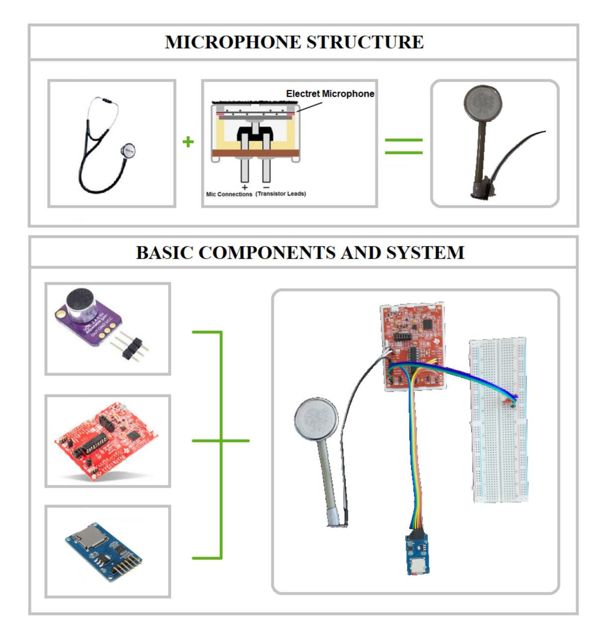
Data are transferred to the computer via an SD card reader. The transferred data becomes readable and processed by Matlab after going through some processes.
