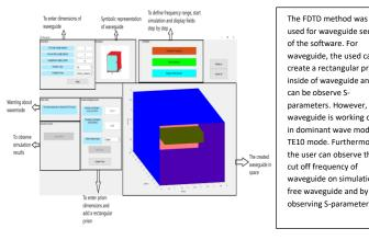
used for waveguide section of the software. For waveguide, the used can create a rectangular prism inside of waveguide and can be observe Sparameters. However, the waveguide is working only in dominant wave mode ie. TE10 mode. Furthermore. the user can observe the cut off frequency of waveguide on simulation of free waveguide and by observing S-parameters.
