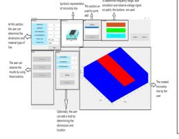
While developing the software for microstrip lines, Finite-Difference Time-Domain method was used. Hence that, the simulation operation take a long time. Furthermore, the software calculates the characteristic impedance of microstrip line and assign the value as port impedance. As the other feature of the software, the user can add a stub and create a microstrip filter.
