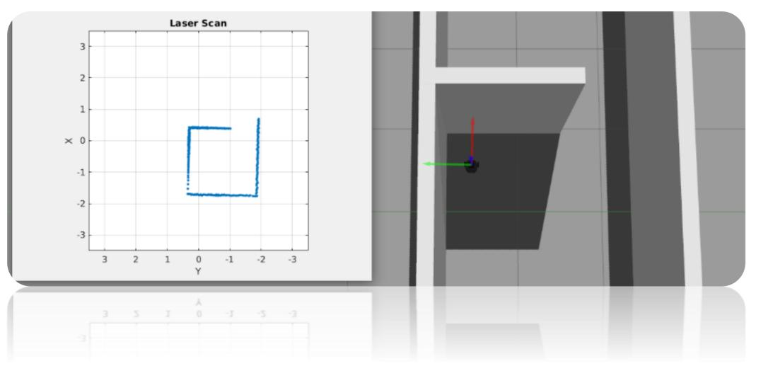
Lidar data was segmented according to distances and angles. The TurtleBot moves according to this data segments.
