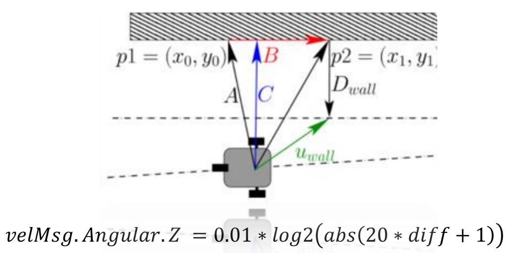
After TurtleBot3 understands that if it is in hallway, checks LIDAR data to find closest point and if closest point's index greater than 180 means referring wall is the right side and makes index 90 with given formula. If index lower
