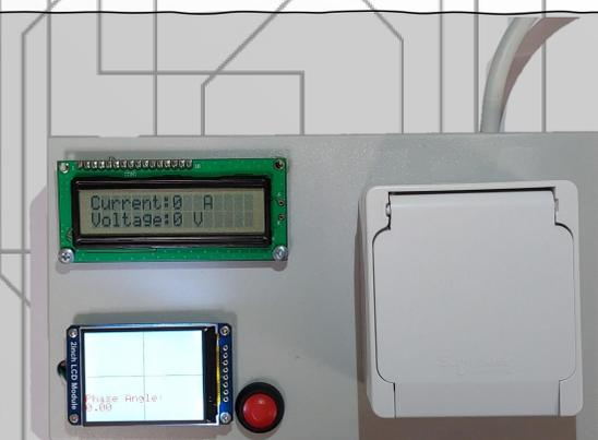
The need for the project was a device that tests measures AC motors and sends the results to the relevant people in various ways. The project was largely successful. Data from sensors can be transmitted to users. However, the phase
