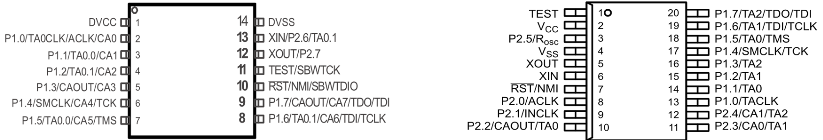
Fig. 3.22 Package pinout of two MSP430 microcontroller models: a MSPG2231 Pin description, b MSP430x1xx Pin description ( Courtesy of Texas Instruments, Inc. )
