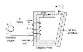
$$\begin{split} \Delta W_{elec} &= \Delta W_{fld} + \Delta W_{mech} \\ \Delta W_{elec} &= \int_{\phi_0}^{\phi_1} \mathcal{F} \, d\phi = A_1 + A_3 \\ \Delta W_{fld} &= \int_0^{\phi_1} \mathcal{F} \, d\phi - \int_0^{\phi_0} \mathcal{F} \, d\phi = \left(A_1 + A_2\right) - \left(A_2 + A_4\right) \end{split}$$
