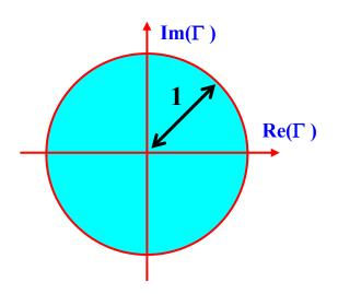
The domain of definition of the reflection coefficient for a loss-less line is a circle of unitary radius in the complex plane. This is also the domain of the Smith chart.
