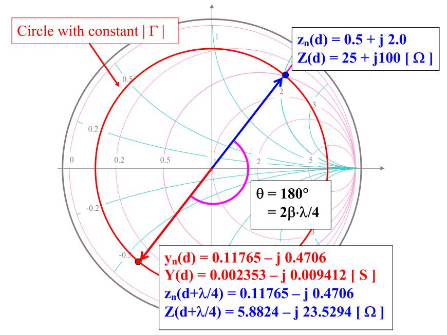
The Smith chart can be used for line admittances, by shifting the space reference to the admittance location. After that, one can move on the chart just reading the numerical values as representing admittances.
