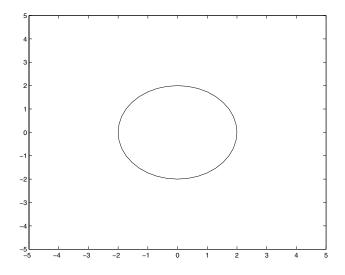
Figure 3.18 Circular data appears elliptical without customizing the axes with the axis command.
