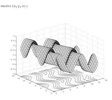
Figure 4.23 Using meshc to create a mesh - contour combination plot.
