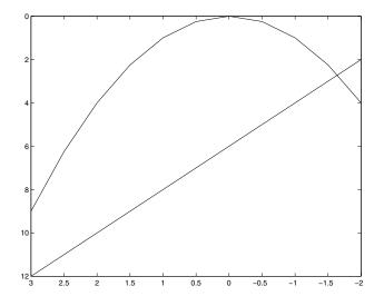
Figure 7.24 Reversing axis direction with XDir and YDir.
