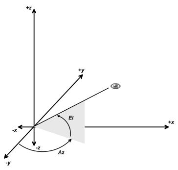
Figure 4.36 The point-of-view in a 3-D plot.
