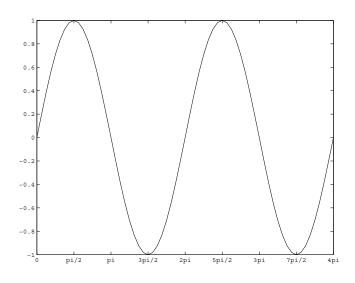
Figure 7.11 Specifying x-axis tic mark labels with XTickLabel.
