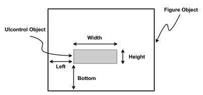
Figure 10.15 The location of uicontrol objects given by Position.
