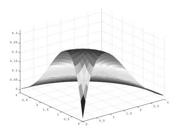
Figure 8.14 Using NaNs to remove unwanted portions.
