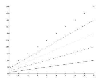
Figure 7.21 Cycling line styles automatically with LineStyleOrder.
