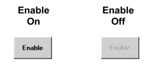
Figure 10.11 Enable property can deactivate a control.
