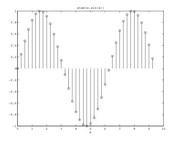
Figure 3.41 Visualizing discrete data with stem.
