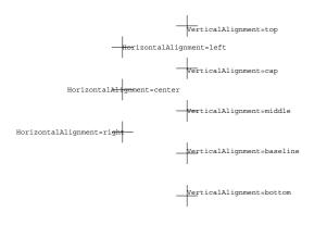
Figure 7.46 Horizontal- and VerticalAlignment properties.
