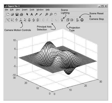
Figure 4.33 The Camera Toolbar in the Figure Window.
