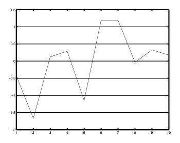
Figure 7.17 Altering the axes' LineWidth and GridLineStyle properties.
