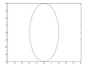
Figure 3.21 Using axis('equal') to graph the ellipse.
