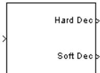
This block performs Walsh demodulation of the combined output of the rake fingers. It outputs soft and hard decision values.
