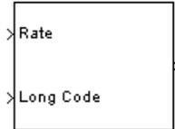
This block generates a pseudorandom masking pattern of zeros and ones. The pattern can be used to mask redundant power groups in a data frame. The data rate and 14 bits from the long code determine the masking pattern.
