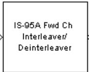
**Inputs** Real vector (of binary data for interleaver functionality) that represents the data frame to be interleaved or deinterleaved. The size of the input is 384 for the Paging and Traffic channels and 128 for the Sync channel.
