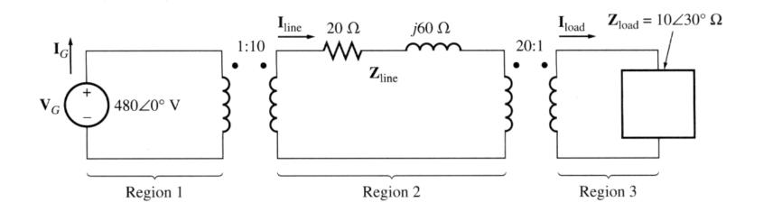
The generator is rated at 480 V and 10 kVA.
