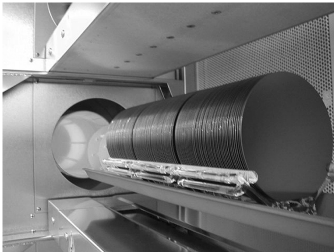
Showing silicon wafers waiting to be pushed into the furnace for device fabrication
