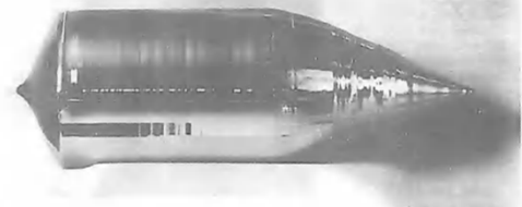
Figure 1-11 Silicon crystal grown by the Czochralski method. This large single-crystal ingot provides 300 mm (12-in.) diameter wafers when sliced using a saw. The ingot is about 1.0 m long (including the tapered regions), and weighs about 1.40 kg. [Photograph courtesy of MEMC Electronics Intl.]
