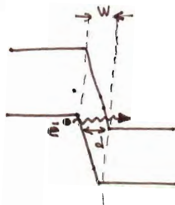
b.) heavily doped junction with rev. bias; electron tunnelling occurs from p to n.
