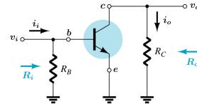
Then, we are going to replace BJT with its common-emitter hybrid equivalent model as shown below
