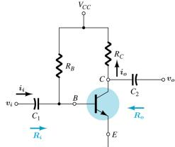
Let us start SSAC analysis by drawing the AC equivalent circuit as shown below
