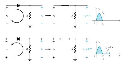
As we see from the figures above, negative half-cycle portion of the signal is clipped off while the positive half-cycle portion remains intact.
