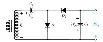
Using the **ideal diode** model, operation of the voltage doubler circuit are shown for the first positive and negative half-cycles the two figures below, respectively. After the first cycle, both diodes retain their OFF state.
