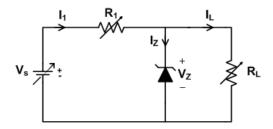
lacktriangle Similarly, we can also write down the equation for  $I_{Z(max)}$
