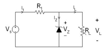
**Example 9:** (2004-2005 MI) In the figure above,  $V_s$  is an unregulated voltage that varies between  $6\,\mathrm{V}$  and  $7\,\mathrm{V}$  while the Zener diode voltage is  $V_Z=5\,\mathrm{V}$ . The load resistor  $R_L$  can have a value from  $100\,\Omega$  to  $\infty$  (i.e., open circuit). Also you can take  $I_{Z(min)}\cong 0\,\mathrm{A}$ .
