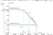
The  $h_{fe}$  parameter (or eta) of a transistor varies with frequency as shown above and given by
