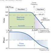
The purpose of frequency analysis in this course is to determine the low-frequency cutoff  $f_L$  and the high-frequency cutoff  $f_H$  of the amplifier. Low-frequency cut-off  $f_L$  is determined by the capacitors in the circuit, i.e.,  $C_1$ ,  $C_2$  and  $C_3$ , and high-frequency cutoff  $f_H$  is determined by the internal device capacitances, wiring capacitances or parasitic capacitances.
