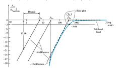
As  $R_{eq_3}$  normally has the lowest resistance value, generally  $f_{L_3}$  holds the highest value. Also as generally  $R_i>R_o$ , mostly  $f_{L_2}>f_{L_1}$ . So, generally  $f_{L_3}>f_{L_2}>f_{L_1}$ .
