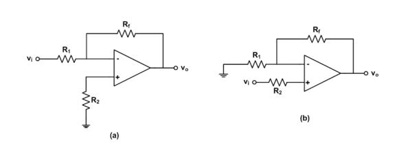
Figures (a) and (b) above show inverting and noninverting amplifiers both with an offset compensation  $R_2$  resistors, respectively.
