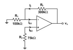
Solution: Let us first show that  $v_o \neq 0$  when  $R_2 = 75 \text{ k}\Omega$ , as  $v_o = R_f I_{IO} = (0.3M)(0.02\mu) = 6 \text{ mV}$ . Thus, the value of  $R_2$  which eliminates the offset is  $R_2 = (R_1 || R_f) \frac{I_{B_1}}{I_{B_2}} = 75k(100n/80n) = 93.75 \text{ k}\Omega$ .  $I_f \qquad I_{B_2} \qquad I_{B_1} \qquad I_{B_2} \qquad$
