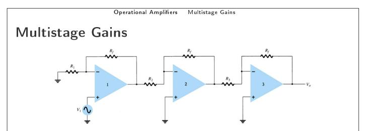
As a voltage-gain amplifier, the input resistance of op-amp amplifiers are high and the output resistances are small. So, when cascaded we can ignore the loading effects and multiply the gains of each stage in order to find overall gain, i.e.,
