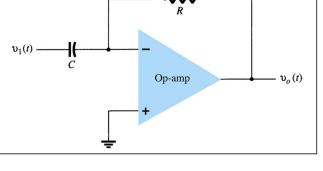
The differentiator takes the derivative of the input. This circuit is useful in high-pass filter circuits.
