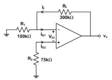
Solution: Let us first show that  $v_o \neq 0$  when  $R_2 = 75 \,\mathrm{k\Omega}$ , as  $v_o = \left(1 + \frac{R_f}{R_1}\right) V_{IO} + R_f I_{IO} = (1 + 0.3M/0.1M)(2m) + (0.3M)(0.02\mu) = 14 \,\mathrm{mV}.$ Thus, the value of  $R_2$  which eliminates the offset is  $R_2 = \frac{V_{IO}}{I_{B_2}} + (R_1 ||R_f) \frac{I_{B_1}}{I_{B_2}} = 25k + 93.75k = 118.75 \,\mathrm{k\Omega}.$
