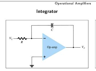
The output is the integral of the input. Integration is the operation of summing the area under a waveform or curve over a period of time. This circuit is useful in low-pass filter circuits and sensor conditioning circuits.
