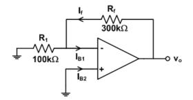
**Solution:** Let us first show that  $v_o \neq 0$  when there is no resistor the non-inverting terminal, i.e., when  $R_2 = 0$ , as  $v_o = R_f I_{B_1} = (0.3M)(0.1\mu) = 30 \text{ mV}$ . Thus, the value of  $R_2$  which eliminates the offset is  $R_2 = R_1 ||R_f = 100k||300k = 75 \text{ k}\Omega$ .
