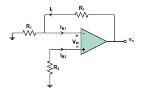
Let us write down the two KVL equations (implicitly using KCL) available in the figure above in order to express output  $v_o$  in terms of the input offset voltage,  $V_{IO}$ , and input bias currents,  $I_{B_1}$  and  $I_{B_2}$  when there is no input present, i.e.,  $v_{i_1} = v_{i_2} = 0$ .
