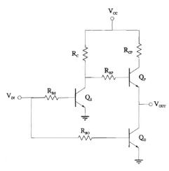
**Example 4:** Compare the maximum fan-out for the RTL inverter with active pull-up with that of basic RTL inverter where  $V_{CC} = 5 \text{ V}$ ,  $R_{BP} = R_{BS} = R_{BO} = 10 \text{ k}\Omega$ ,  $R_C = 1 \text{ k}\Omega$ ,  $R_{CP} = 100 \Omega$ ,  $V_{BE(SAT)} = 0.8 \text{ V}$ ,  $V_{CE(SAT)} = 0.2 \text{ V}$  and  $\beta_F = 25$ .
