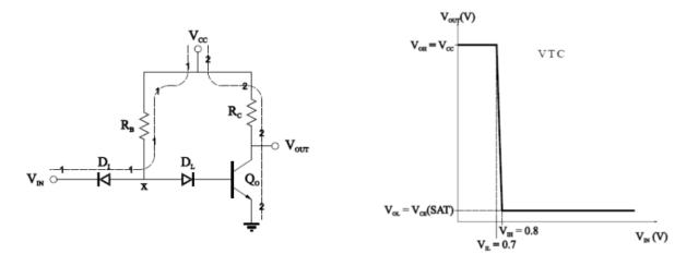
A basic DTL inverter and its VTC are shown in the figure on the left and right above, respectively.
