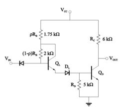
The states of active elements in a transistor modified DTL inverter are given in the table below.
