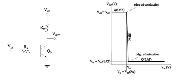
A basic RTL inverter and its VTC are shown in the figure on the left and right above, respectively.
