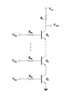
**Example 1:** For the basic RTL NAND gate above, determine the maximum fan-in if all stack BJTs have  $V_{CE(SAT)} = 0.17$  V and all load gates have  $V_{BE(FA)} = 0.7$  V.
