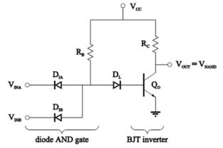
Example 5: Consider the DTL NAND gate in the figure above, and determine
