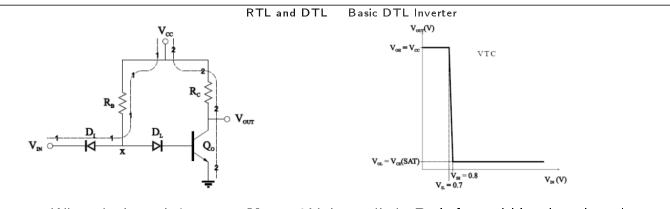
• When the input is low, e.g.,  $V_{IN} = 0$  V, input diode  $D_I$  is forward biased so the voltage  $V_x$  between the diodes will be  $V_x = V_{IN} + V_{D,I(ON)}$  and thus as  $V_{BE,O} = V_x - V_{D,L(ON)} = V_{IN}$ , output transistor  $Q_O$  will be in **cutoff** mode. Consequently, output is HIGH as  $V_{OUT} = V_{CC}$  (because  $I_C = 0$ )
