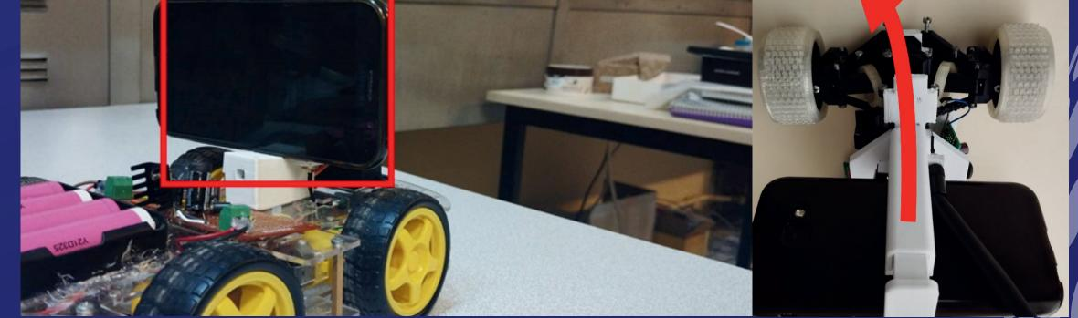
Figure 3: Tracking Mode Inference GPS & LiDAR based driving uses the mapping created by using the external LiDAR module and needed bearing and distance to reach the target location.
