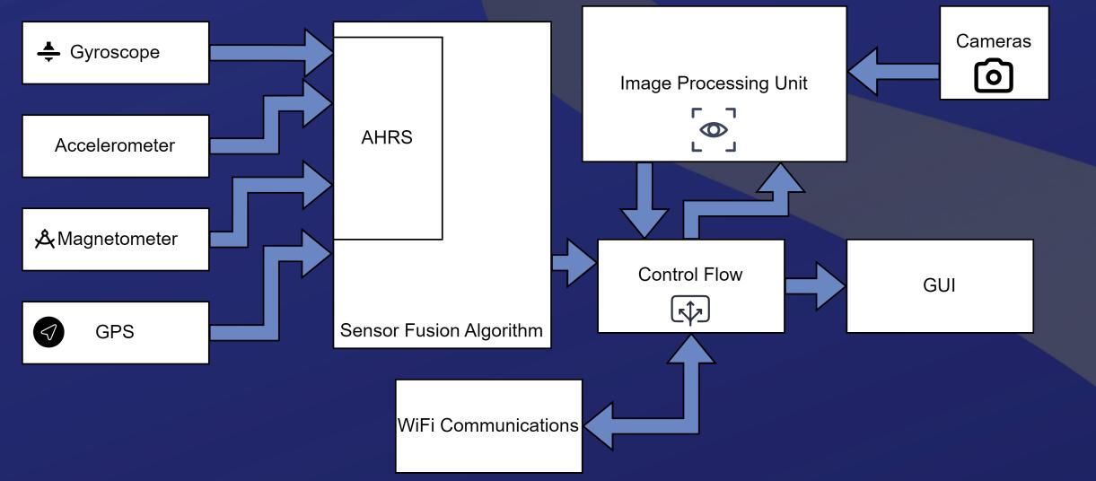
Figure 1: Smartphone Software Architecture With such capabilities the older devices can gain a new meaning as robot controllers and newer devices become cutting edge robotic development platforms that can be used in exploration, search and rescue or autonomous food delivery systems.
