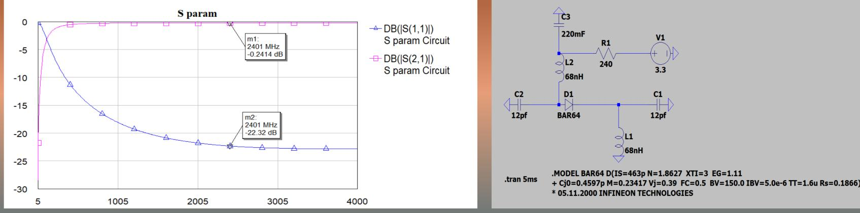
Forward Voltage Gain: When we examine the S21 parameter values of the circuits we designed, we can observe that there are quite good values in the desired frequency band. Biasing Circuit: The consideration of DC biasing parameters ensures that the pin diode operates effectively, exhibiting behaviors such as current-controlled resistance and high impedance for RF signals as intended.
